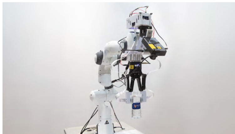
The novel robotic system developed by NUS researchers comprises an artificial brain system that mimics biological neural networks and which can be run on a power-efficient neuromorphic processor such as Intel's Loihi chip, and is integrated with artificial skin and vision sensors. Image: National University of Singapore.
