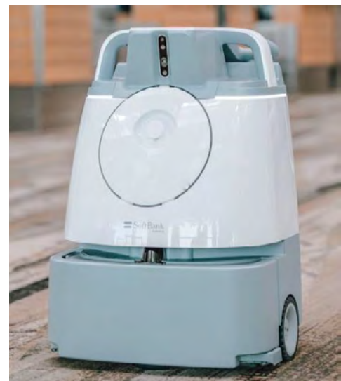
Autonomous cleaning robots used in Changi Airport’s terminals have been equipped with a misting attachment that disinfects the carpets immediately after cleaning. This is in addition to daily carpet vacuuming undertaken by a separate set of cleaning robots equipped with a HEPA filter that catches fine particles while vacuuming. Photos: Changi Airport Group
