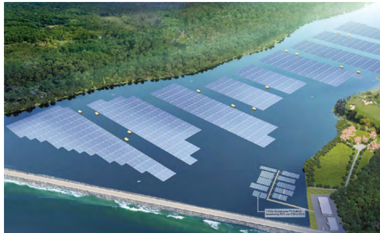
Artist's impression of the upcoming 60 MWp floating solar PV system on Tengeh Reservoir, that will occupy an area of about 45 football fields.
