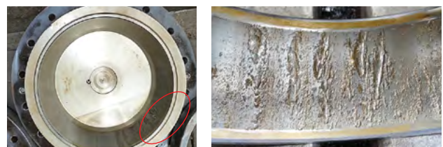
Spalling on the running path pattern of the outer ring of the tapered roller bearing.
