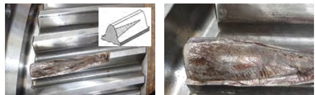
Broken tooth of input pinion. The cracking was initiated under the case hardened layer and it then propagated parallel with the tooth flank.
